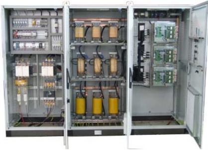
Figure 8. Proposed up to 135 kVA micro-grid converter
